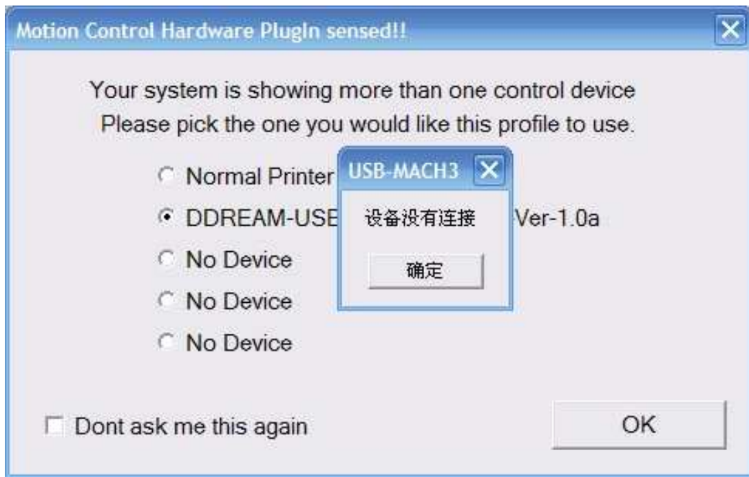
Figure4-2. Not connected correctly
